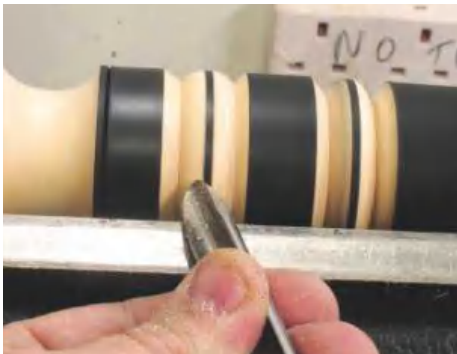
▲ Pic.9 Cutting a bead with the gouge is very similar to cutting one with a skew, but because of the angle of the bevel, this won't give you a narrow cut to the side
